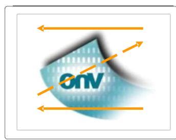
Fig. 2 Reverse scan (Pin19, REVERSE = High)
