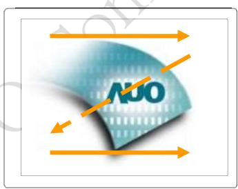
Fig. 1 Normal scan (Pin19, REVERSE = Low or NC)
