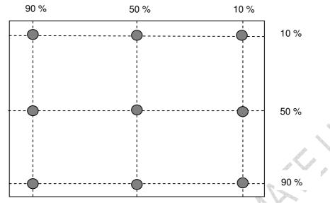
Note 3: The luminance uniformity of 9 points is defined by dividing the minimum luminance values by the maximum test point luminance
